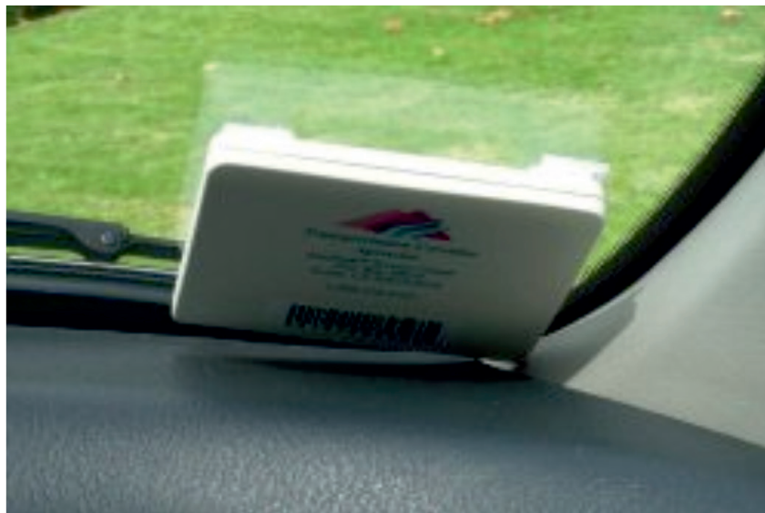
Image 2. An RFID tag used for electronic toll collection
